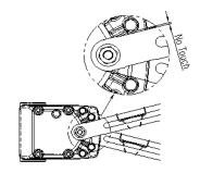
8 After the proper installation, tighten all of the bolts on the bracket, the feedback lever, and the connection bar.
